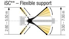
Dimensions can differ depending on configuration. Support width based on center of support leg. Diameter of swivel plate 270 mm.
