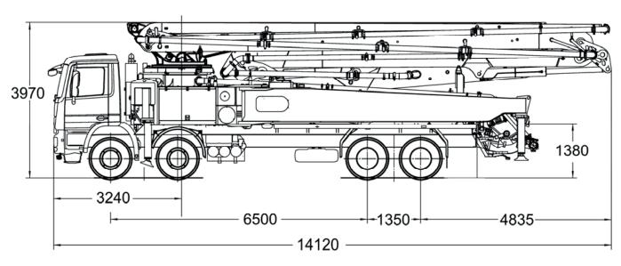
Note: Standard version. Dimensions and weights depend on truck, pump model and equipment. Dimensions in mm, MB-Actros 4640 B, Euro 2.
